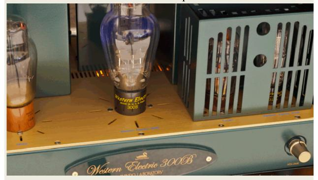
The legendary Shindo Western Electric 300B Limited Mono Block Amplifier. Ken Shindo designed his first 300B single ended amplifier in 1979. Continually refined over the years, the WE 300B Single Limited is the flagship Shindo amplifier. Genuine NOS Western Electric 300B tubes from the original production run are employed for 8 watts Class A output. Speakers of 90db sensitivity or higher are recommended.
